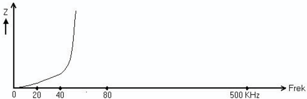
Gambar 5.47 Kurva Impedansi Drain Coil
