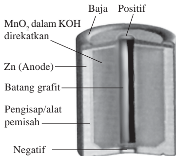
Gambar 2.4 Baterai Alkaline. Sumber: Chemistry, The Molecular Nature of Matter and Change, Martin, S.Silberberg, USA
