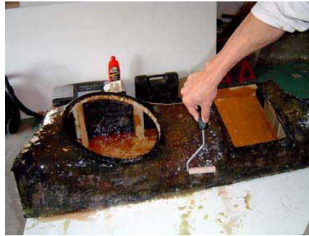
Gambar 12.9. Adonan Fiberglass diratakan
