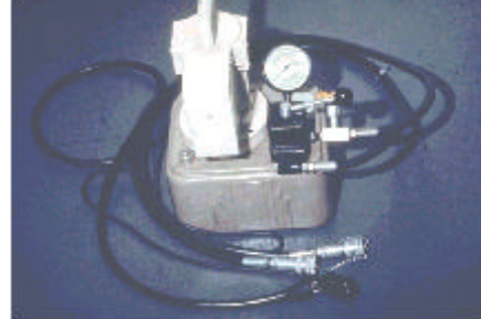
ELECTRIC HYDRAULIC PUMP
