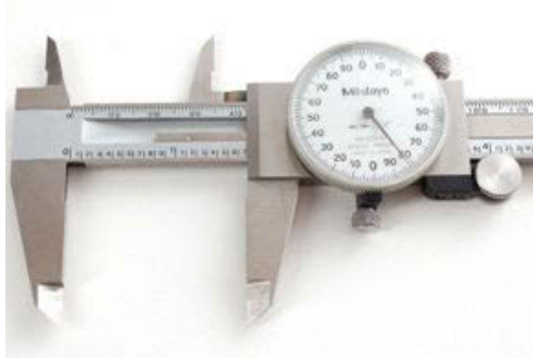
Gambar 1.27. Dial Vernier Calliper
