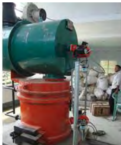
Twin Chamber, Pyrolytic & Controlled Air Incinerator
