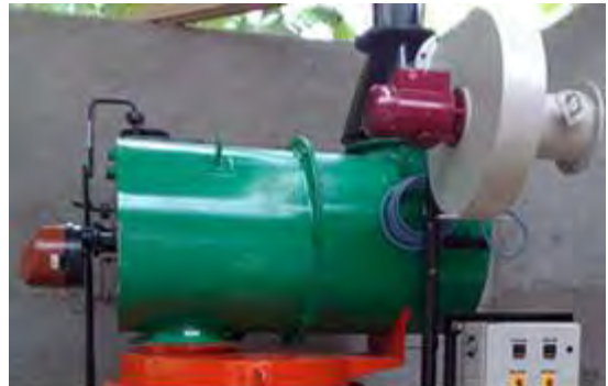
Secondary Combustion Chamber
