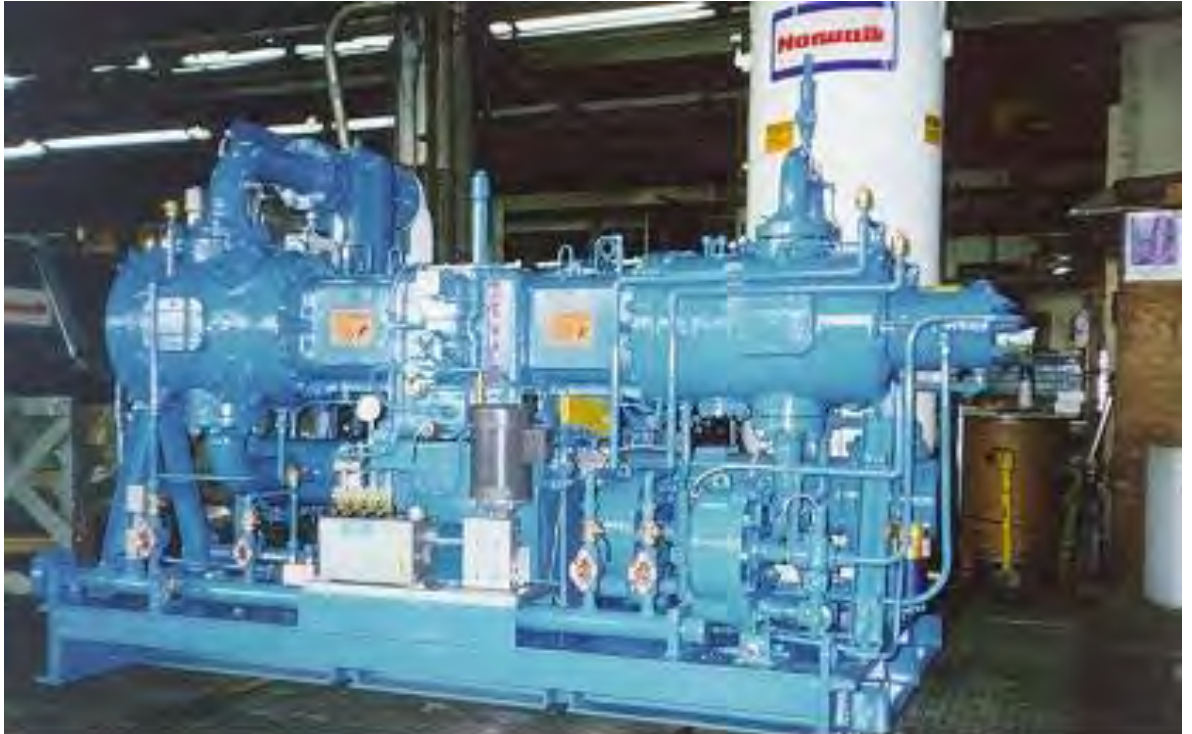
Norwalk "Century Series", Horizontal, Balance Oppose, Three Stage, Two Throw
