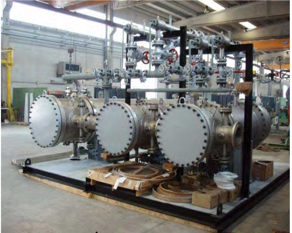
GAMBAR : 3 – 5 HEAT EXCHANGER
