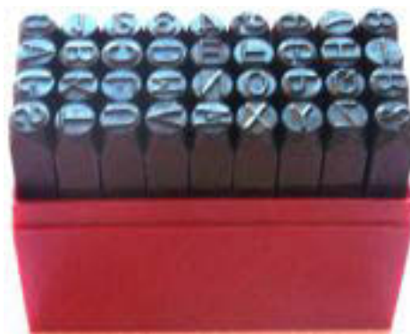
Gambar 7.17 Stempel Baja ( Steel Stamping )
