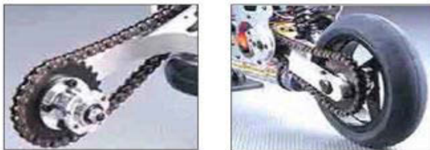
Rear wheel chain drive of a motorcycle
