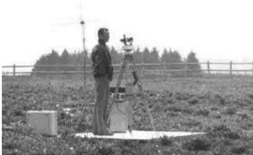
Gambar 5. Alat ukur theodolite
