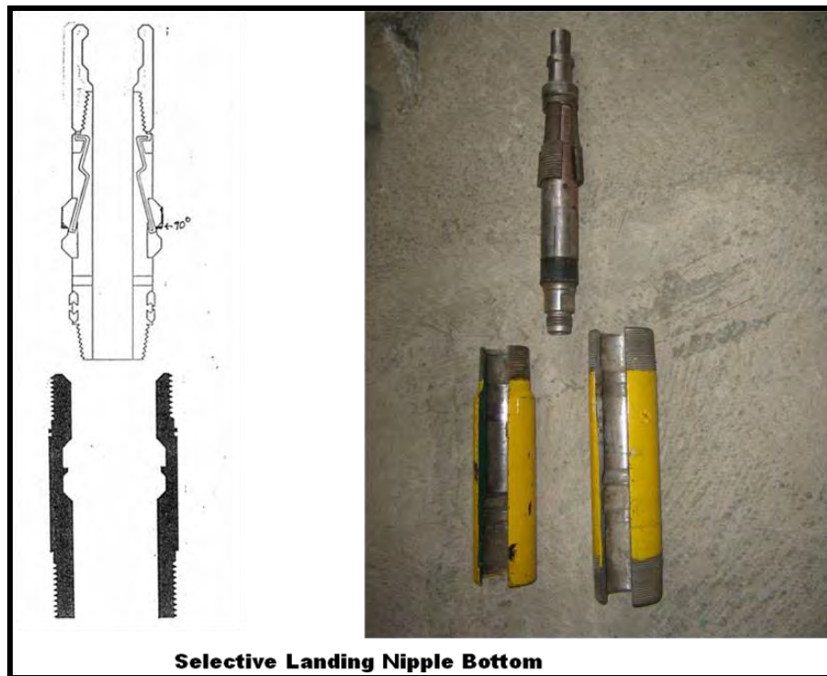
Gambar: 8 Selective Landing Nipple
