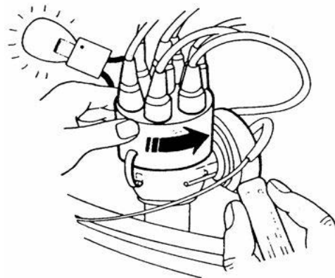
Gambar 16.8 Putaran distributor berlawanan arah jarum jam
