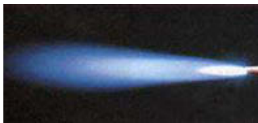
Gambar model Api Carburizin
