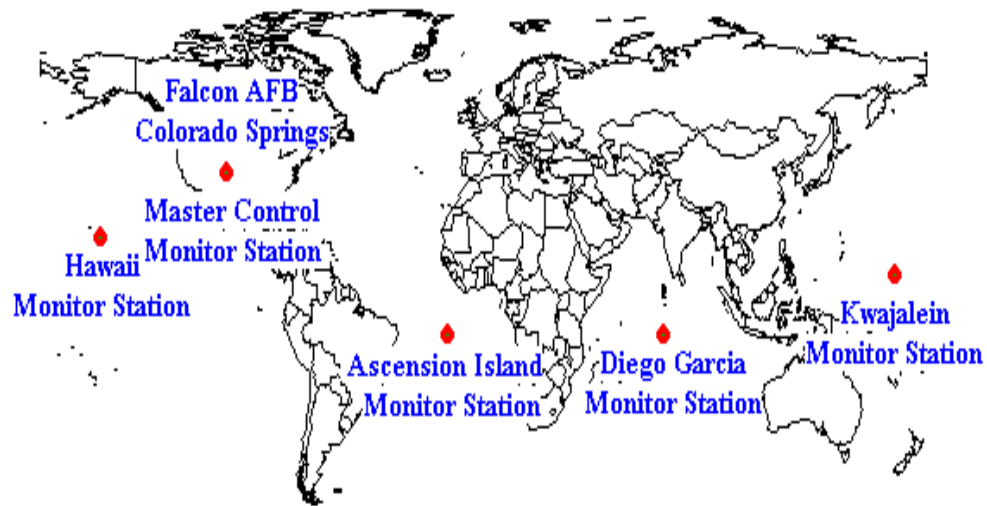
Global Positioning System (GPS) Master Control and Monitor Station Network
