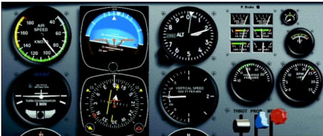
Figure 11-5. Vacuum failure—inoperative attitude and heading indicators.
