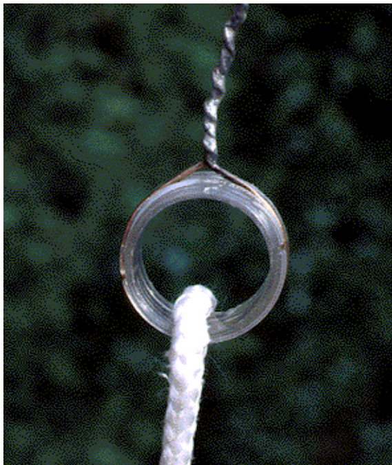
A bottleneck antenna insulator.
