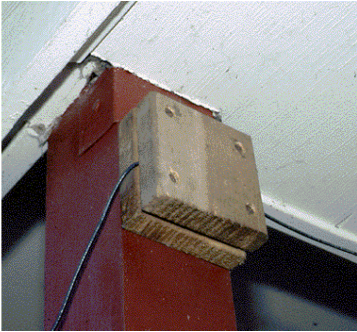
A wooden-block longwire clamp.
