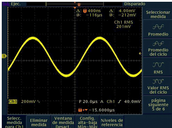
Figure 15: Signal at TP8 after adjusting the left input trimpot. The other channel looks exactly the same.
