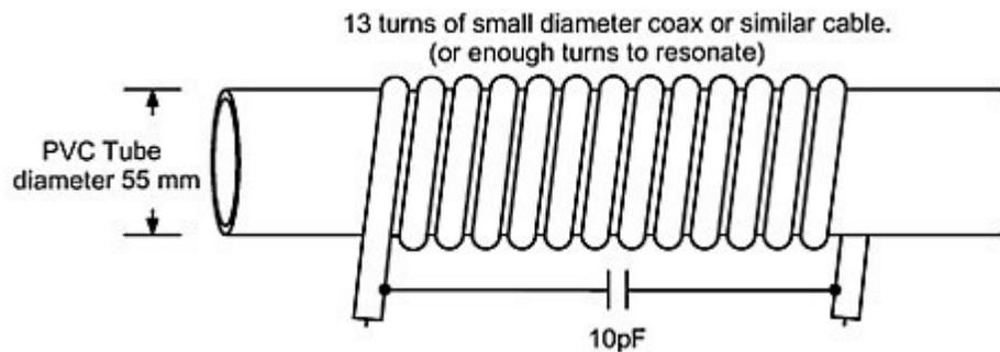
**Figure 8 - 20 Metre Trap, Air Core**
