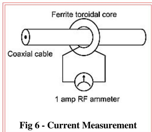
**Fig 6 - Current Measurement**
