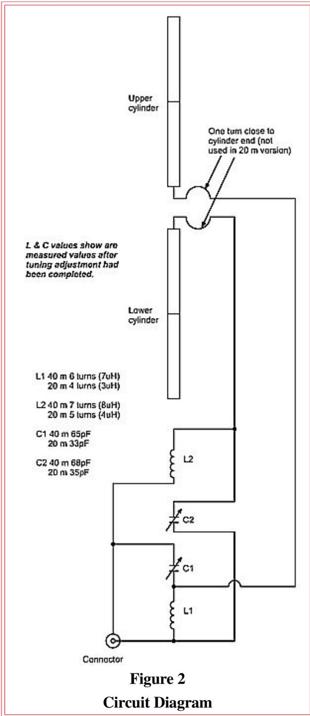
Ted Hart discovered that if he introduced a phase shift (in fact 90 degrees) into the circuit feeding the EH dipole cylinders, the radiation dramatically increased, resulting in increased series radiation resistance (or equivalent reduction in the equivalent parallel radiation resistance). This was incorporated into reactive networks designed to match the new reflected antenna impedance to a 50 ohms source. The typical L+L matching network is shown in figure 2.
