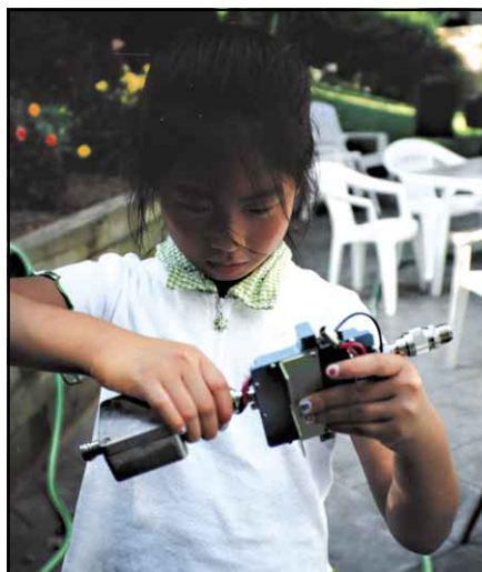
Putting together a 2.4-GHz receive system is child's play—literally. My daughter attaches a preamp to a modified Drake downconverter in preparation for another OSCAR 40 session.
