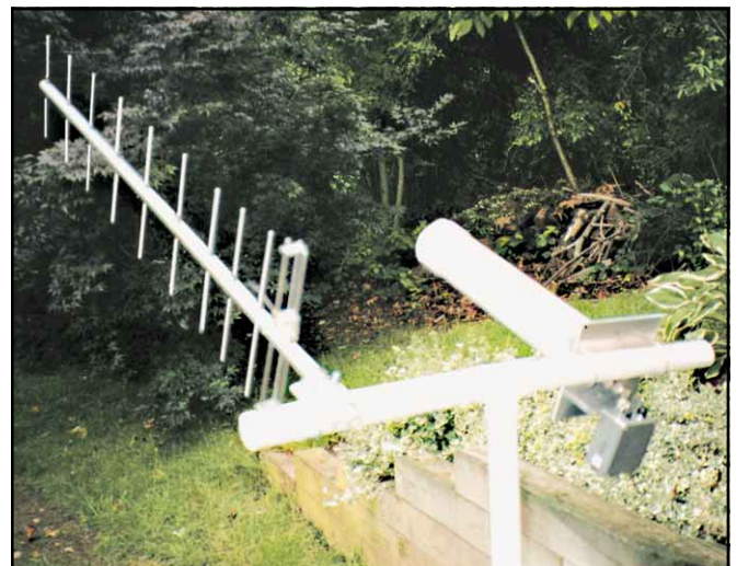
This is yet another incarnation of my OSCAR 40 antennas, this time using the Down East Microwave helical antenna (the glaringly white plastic tube aimed at the heavens). I find that I achieve somewhat better performance from the dish, but the helical antenna does an adequate job—especially when I have the 2.4-GHz preamp in the line.
