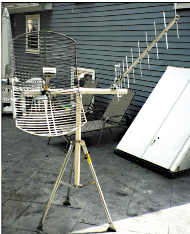
My portable OSCAR 40 antenna system with the barbecue grill dish attached. The tripod was purchased at RadioShack and the PVC is courtesy of my local hardware outlet. I can set up my antennas in about 15 minutes.
