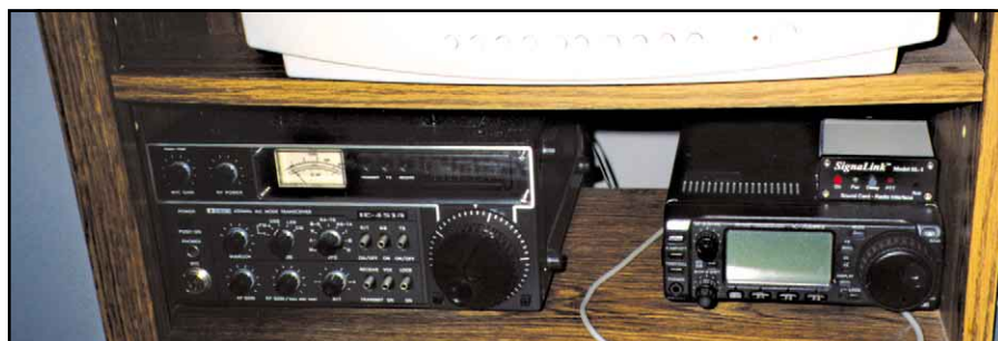
The "shack end" of my OSCAR 40 station. At the left is the IC-451 all-mode 70-cm transceiver. My IC-706 transceiver (right) serves as the microwave receiver. I can operate from this desk or, when the spirit moves me, I can drag everything out to the patio for a little "satellite al fresco ."
