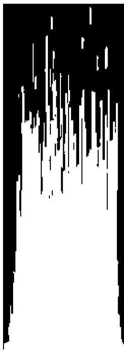
A typical analogue channel, this one was Channel 4 at 823.25MHz with a sound carrier (right) at 829.25MHz
